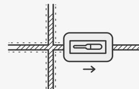
The grouting material should be applied with a rubber trowel (using metallic trowels may damage the glazed surface of tiles). We recommend that you use the most suitable grouting material colour to match the floor or wall cladding.
