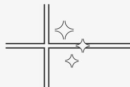
The installation joints must be empty and free of bonding materials and traces of dirt and grime. In this way, the adhesion of the grout will be improved and will be more effective.
