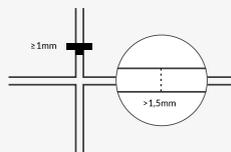
According to "The Ceramic Tile Guide", the separation between pieces must be more than 1.5 mm. The cross-spacers to be used must be at least 1 mm.
