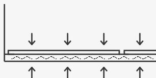
Joints should be grouted once tiles are firmly bonded to the substrate (please check adhesive manufacturer's recommendation).
