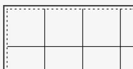
We recommend that you consider the inclusion of perimeter joints, which will help absorb any movements after installation. If the substrate already has its own structural joints or dividing joints, these must be respected when ceramic tiles are installed.
