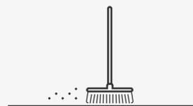
For better bonding strength of the adhesive we recommend first cleaning the surface to be tiled.
