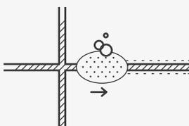
Removing excess grouting material must not be left for too long after finishing the work. Use a sponge dampened in water. This operation will help prevent the grouting material from becoming embedded in the glazed surface, especially in those which has textures some designs of the TECHLAM® collections.
